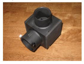
After inserting the end caps, the beam splitter is ready for operation.
