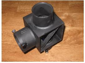
One can have more than one optical insert, and can change it as desired to suit different projects or different telescopes (such as a straight through GEM versus a 90 degree fork).
