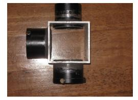
The ends of the Orion extension tubing were ground down slightly to provide a tapered press fit into the square tubing holes. The three extension tubing pieces were placed in a freezer while the square tubing was placed in the sun. A press fit was then made in a vice and JB Weld applied to the seams both inside and out. This was probably total overkill but it is certainly Hell for stout ©.
